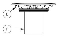
Insert the cup and trap (F&G). Push down firmly to ensure the trap is in the the bottom position.
