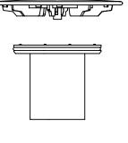
This waste provides a flow rate greater than 24L per minute under a 15mm water load. The flow rate can be seriously impaired if an adequate fall is not maintained throughout the length of the waste pipe.
